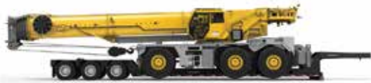
The new RT 9165 is said to be easy to transport on a beam trailer with an overall travel height of 4.23m.
