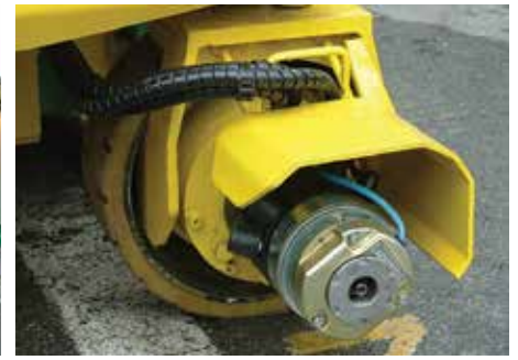
The Iteco IT7380 was the first to follow JLG with direct electric drive.
