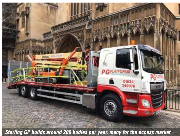
Upward Powered Access' DAF CF 8x2 fitted with Sterling GP access specification beavertail plant body
