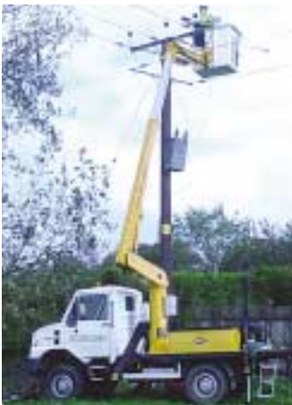
An insulated platform mounted to a Bremach chassis.
