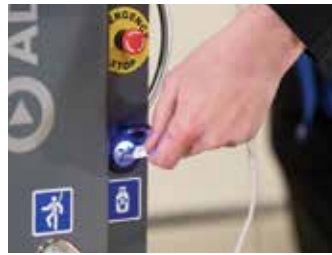
The Safelift's harness anchor point is mounted on the side of the mast just below the emergency stop button and a 12 volt USB socket for charging a tablet or mobile device.
