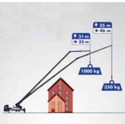
The Klaas K1100 RSX can lift 350kg at a radius of 46m and height of 31m.
