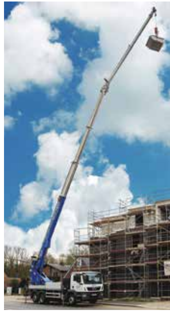
The new Böcker PK 350-D can accommodate up to three people or 350kg
