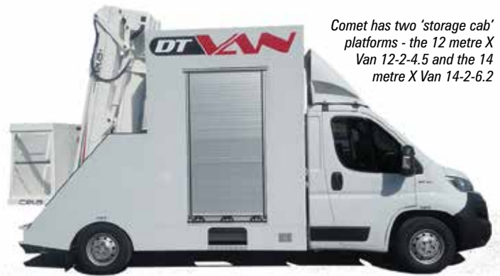
The Comet X Van has a 10 cubic metre storage compartment and can carry up to 300kg of materials or tools
