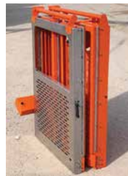
The basket can be folded for stowage or transport.
