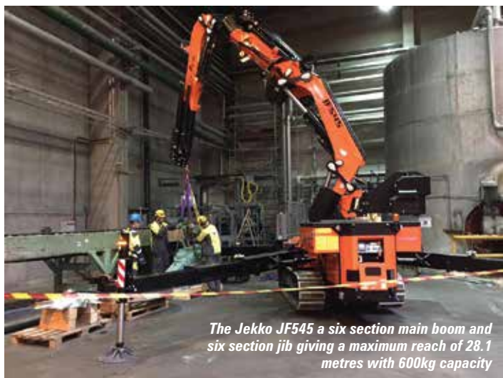
Palfinger is set to unveil three new heavy duty, high capacity PCC tracked articulated boom spider cranes later this month
