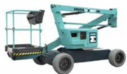
The new lithium powered Nifty HR12 weighs just 2,500kg.
