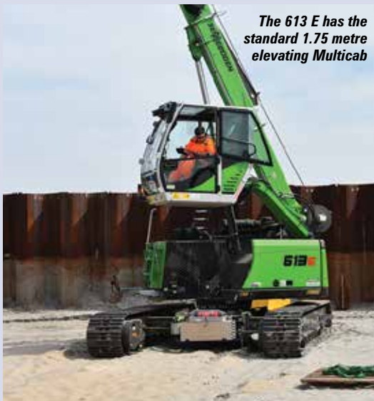
The smallest Sennebogen telescopic crawler crane 613 E is used in Vlaardingen to suspend anchor rods in coffer dams
