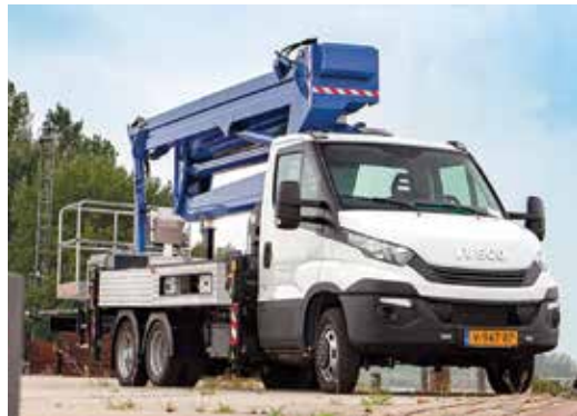
The 31 metre Comet Compact 3117 Jib uses a 3.5 tonne Iveco chassis with the platform mounted on trailer frame that creates a third axle.
