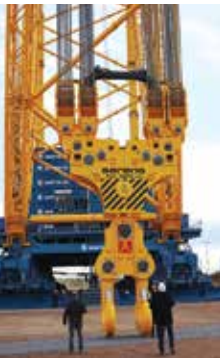
The cranes 3,200 tonne hook block.
