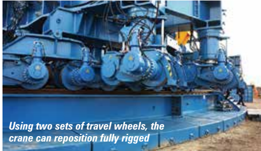
The slewing bogies travel around the ring track
