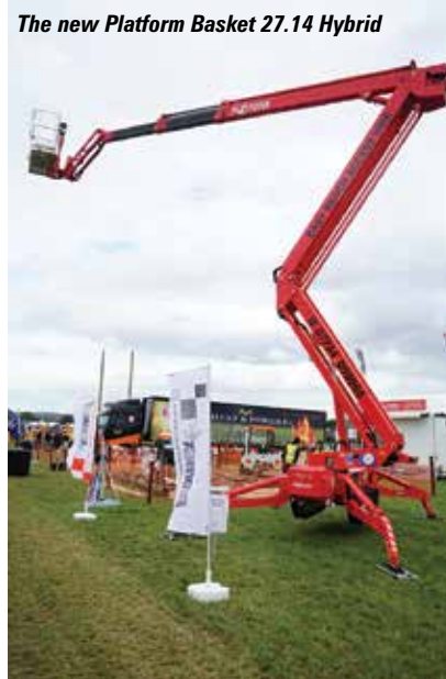
Promax modified Platform Basket 27.14 undercarriage specifically for rental company Easy Reach Access Hire
