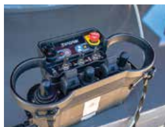
The remote lower controller.
