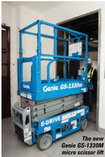
The new model features direct electric drive
