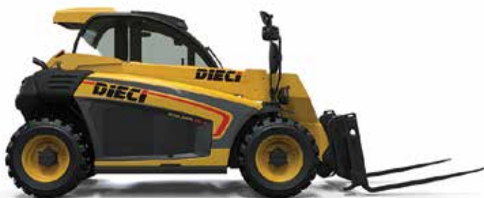
The new Dieci Agri 20-4 is has an overall width of 1.55 metres, is 1.91 metres high and 3.63 metres long.
