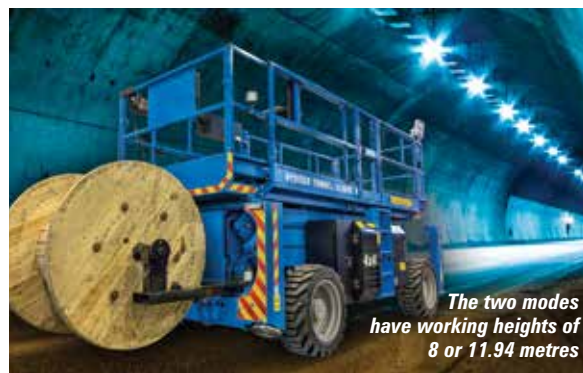
The Hybeko Tunnel GS-3390 includes a chassis mounted cable drum stand
