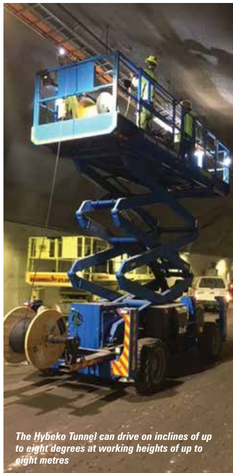
The Hybeko Tunnel GS-3390 includes a chassis mounted cable drum stand
