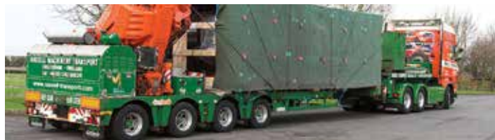
A crane mounted to the rear of a semi trailer offers greater torsional stability and self-weight and is more suitable for bigger cranes.
