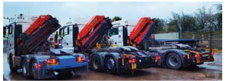
The Broshuis extender neck was found to have high torsional stiffness - well suited for mounting the crane
