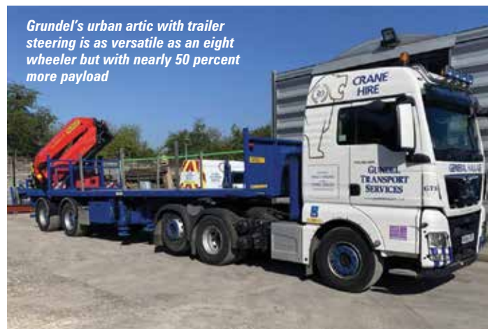
With light bulky loads a forward fitted crane frees up load space
