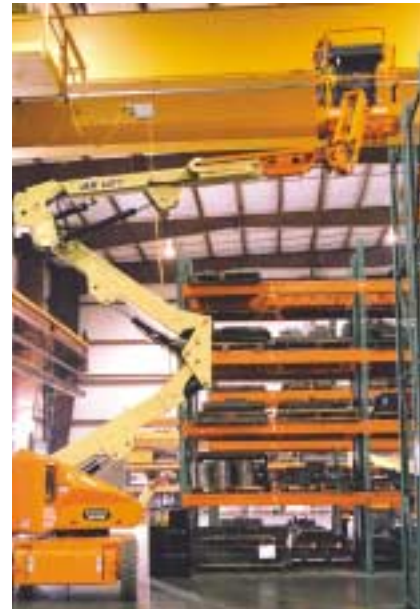
40/45 ft articulated booms are widely used, note the rotating jib
