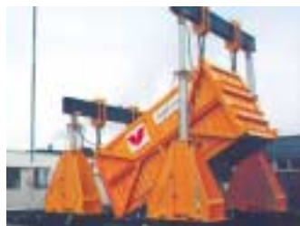
Telescopic lifting gantries are highly versatile for industrial moving.
