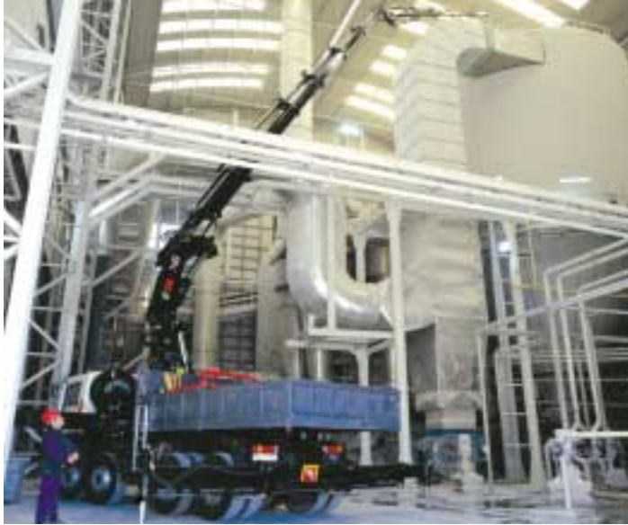
A rare use of a full lorry loader working in plant, they are usually mounted to special chassis for such jobs.
