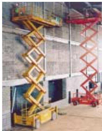
The biggest scissors are ideal for some applications, here a 19m Holland lift (red) and 22m Liftlux
