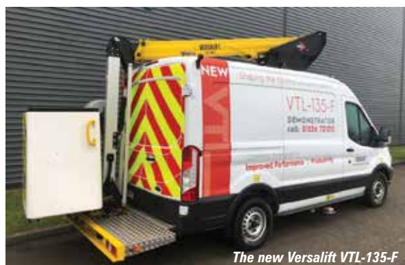
Versalift has developed an all-electric van without stabilisers
