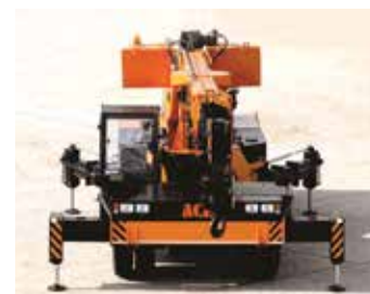
The addition of four outriggers allows it to double up as a 360 degree slewing crane.
