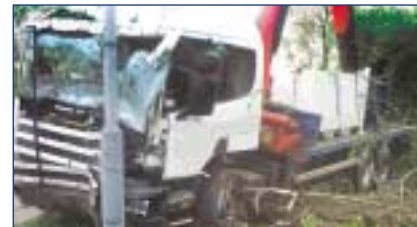
In this incident the driver was in a hurry and said he forgot to put the crane in the transport before leaving the site... He hit the bridge at 56mph and both front tyres blew out causing him to loose control, skidding down the road to it's final resting place.
