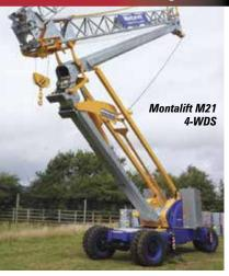
Netherlands-based mobile tower crane manufacturer **Montarent Bouwlogistiek** will bring the **Montalift** M21 4-WDS selfpropelled, self-erecting tower crane which features a Potain tower crane superstructure and an all wheel drive chassis. The 21 metre/tonne crane has a 26 metre jib with a lifting height from 18.7 metres to a maximum of 25.9 metres. Maximum capacity is 1,800kg.
