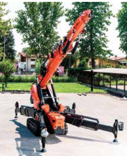
The angle of the beams and the amount of beam extension is completely variable.
