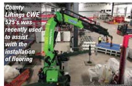
The compact dimensions and variable outriggers allow the CWE 525 to set up within the steel work
