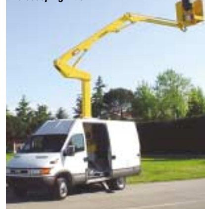
The Skyking 140 MRA with telescoping mast.
