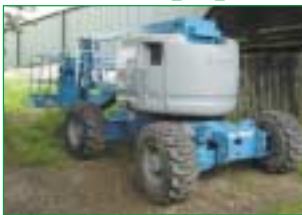
SELF PROPELLED TELESCOPIC PLATFORM 2002 GENIE Z45/22 4x4 15m. working height (46ft.). Oscillating axle. Deutz Diesel. Choice of 5 machines.
