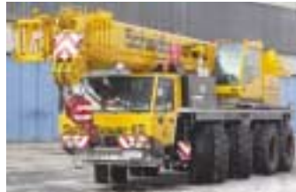
The Tadano-Faun ATF 80-4 with Schaad outrider tyres
