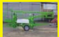
NIFTYLIFT 120HE (1998) Trailer mounted platform. Hydraulic jacks. 40' working height. Battery. Repainted, serviced & tested.
