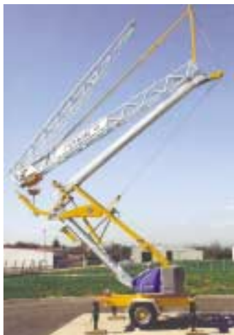
The Potain Igo 13 demonstrates just how fast the smallest self erectors can set up.
