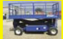
UPRIGHT SL26 (1990) Self propelled scissor lift. 32' working height. Diesel. 4wd Recently repainted, serviced & tested.
