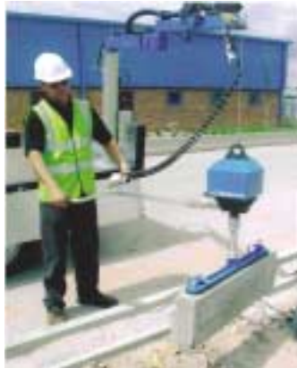
The Al Vac Handy Vacuum kerb lifter is self contained and is hook mounted.
