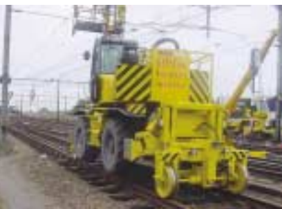
The VHS ManiRail designed for intensive rail maintenance
