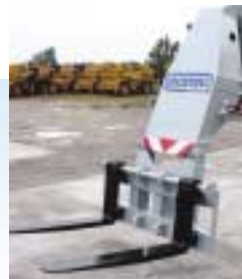
The ATC 20 fork head which also takes an integrated work platform
