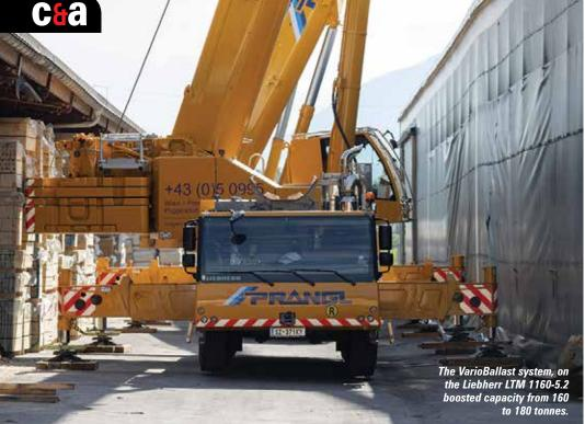
cheeks to be extended rearwards, boosting the crane's capacity, or folded into the crane for reduced tailswing.
