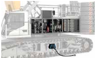
The Unplugged cranes can be recharged from 32, 63 or 125 amp supplies.
