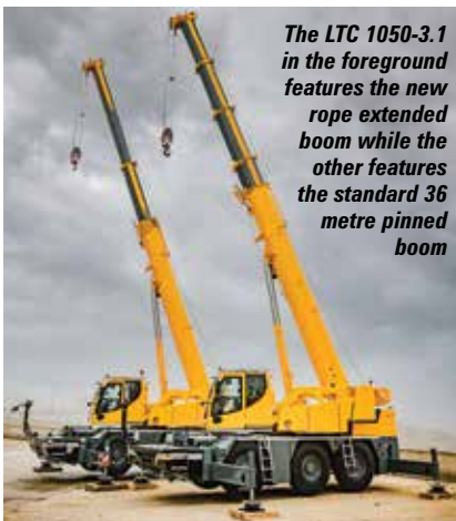
The new 31 metre rope extended boom system
