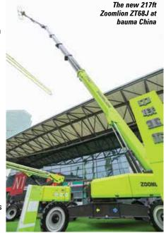
drive speed, 40 percent gradeability and 360 degree continuous slew with a 2.15 metre tailswing. The chassis has swing out legs which is now standard on big booms, while four wheel steering and drive are standard.
