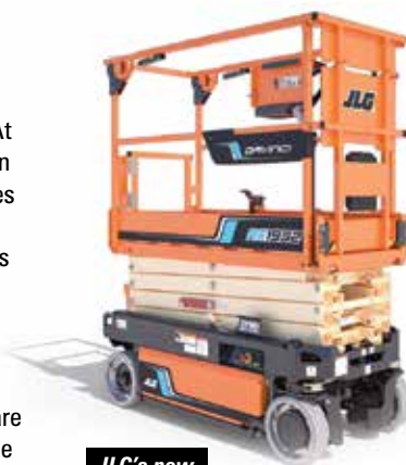
JLG's new AE1932 has no hydraulics
