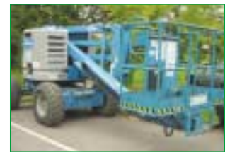
SELF PROPELLED TELESCOPIC PLATFORM 1998 GENIE Z45/22 15m. working height (39ft.). Deutz Diesel Choice of 20 machines.
