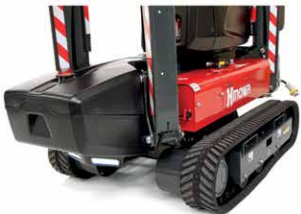
STABILIZATION PLATES HOLDER AND LED FRONT AND REAR WORKING LIGHTS
