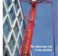
Just as Liebherr's MK range compares with that of Spierings for lifting capacity, so both ranges are designed for rapid set up, with the crane ready to go in under 30 minutes: 10 to 15 minutes to set up the crane on outriggers, and then a similar length of time to fully erect the tower and jib. Set up is not only fast, but fully automated - no assist cranes or helpers.
