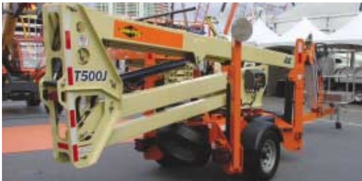
"The all new JLG T500J "Tow Pro" 17 metre trailer lift seen for the first time Conexpo"
