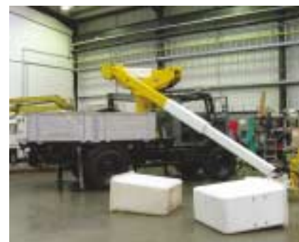
Versalift carry out regular rebuild and recertification of insulated booms
