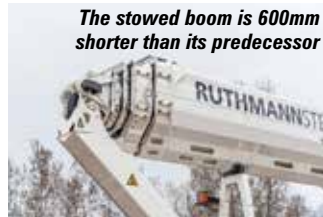
Ruthmann claims the T 300 XS is the most compact 30m on a 7.5t chassis
