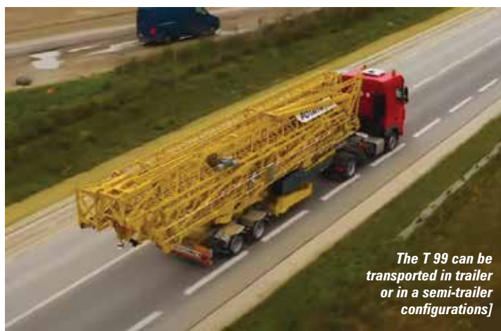
The T 99 offers a 48m jib length with a 38.5m under hook height
