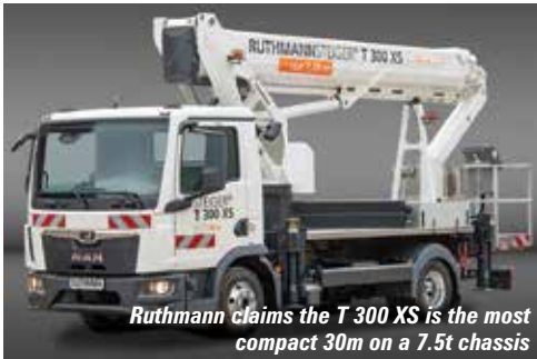
The stowed boom is 600mm shorter than its predecessor
