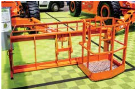
The new Operator Station is attached directly to the fork carriage allowing the operator to ride with the load
