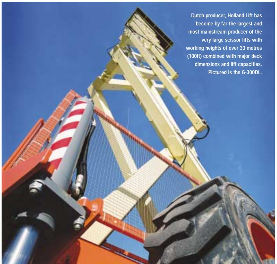
Dutch producer, Holland Lift has become by far the largest and most mainstream producer of the very large scissor lifts with working heights of over 33 metres (100ft) combined with major deck dimensions and lift capacities. Pictured is the G-300DL.
