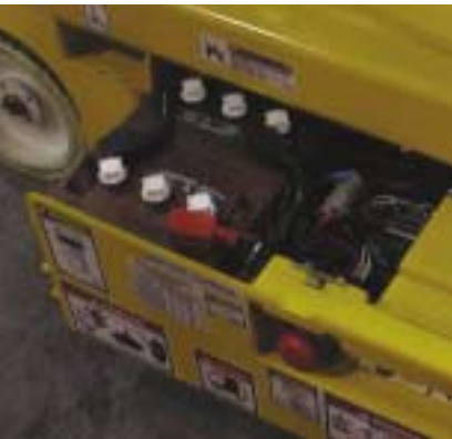
The most common battery in use on aerial lifts today is the six-volt, 220-amp/hour deep-cycle unit.
