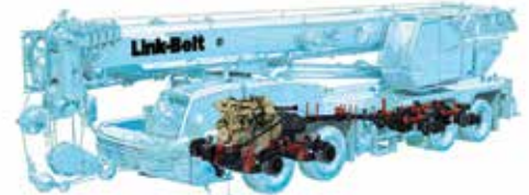
The new drive train and suspension system
