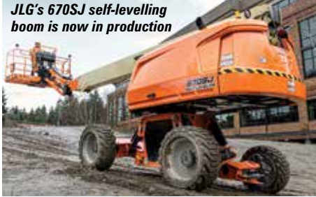
The machine's independent self-levelling system in action
