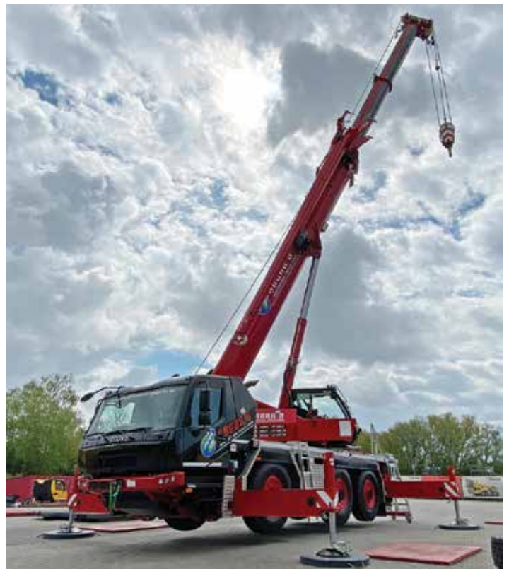
The new Tadano AC 4.070L-1 carries more counterweight within 12 tonne axle loads than any other 60 to 80 tonne AT
