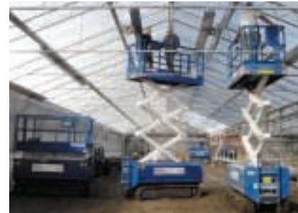
The largest market in Europe for heavy-duty, full width aerial lifts is The Netherlands, where glass house construction on reclaimed polder land is big business.
