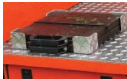
Outrigger pad provision and stowage on a Bison 3.5-tonne truck-mounted platform, now part of the Palfinger portfolio.
