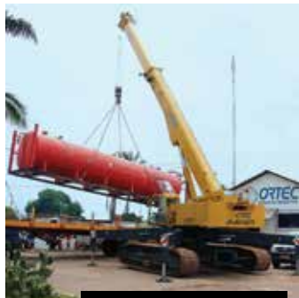
Marchetti's largest model, the CW 70.42L Sherpa, can be levelled on outriggers
