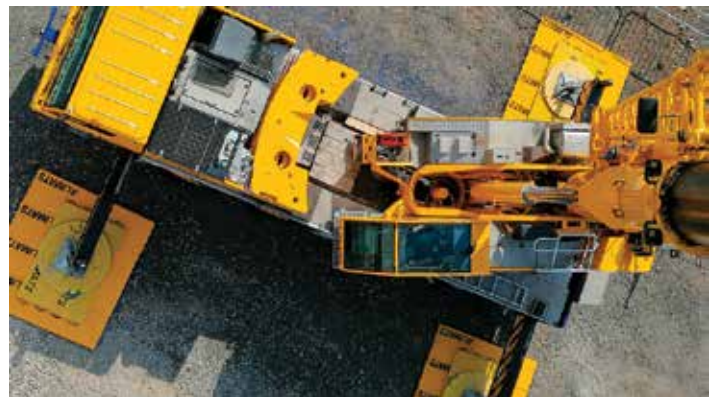
A new Dingli BT24ERT lithium boom lift from Clements and a Demag AC60-3 from Aba Crane Hire working on Warwickshire's Chesterton Windmill using aluminium trackway panels to gain access
