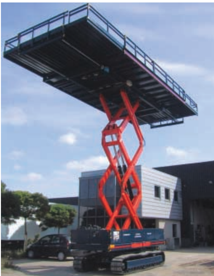
Mega scissor lift: The two-tonne capacity HTN with a dual extension 12- by 5-metre deck and side scissor stack rotation.
