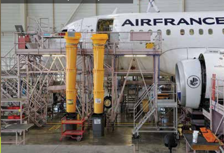
An Airbus 320 surrounded by a nose access dock - note the engineer on the roof is secure being tied in to an overhead fall protection system
