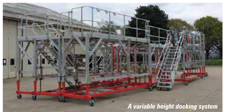
Mobile staging is used when carrying out more in-depth maintenance and repairs
