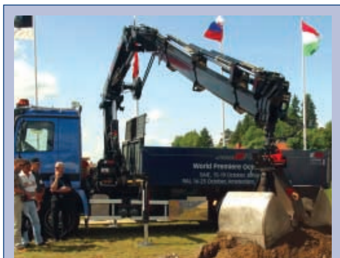
Hiab extended its XS-Series knuckle boom range spanning from five to 76 tonne/metre units. The smallest, the 11.4-metre outreach XS 055, targets middle-weight trucks, while the at the other end of the scale is the XS 800, which features Hiab's integrated computerised Space 5000 operating system. Pictured is the XS 288.
