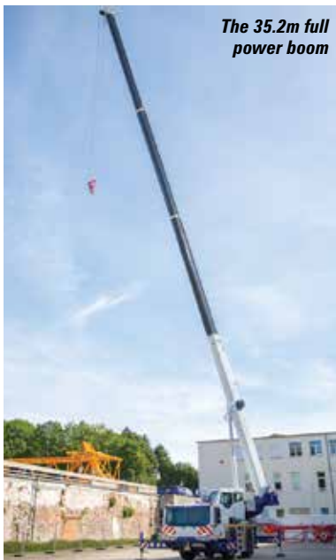
The 6103E can pick & carry its full load chart
