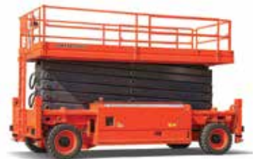
The diesel JCPT3225RT has the same performance as the DC but is 500kg lighter
