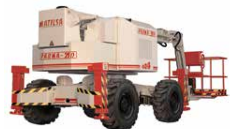
Matilsa Parma 21D can automatically level on its outriggers
