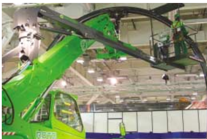
Merlo's new tunneller project is a special extension that grips the tunnel-lining frame, while a boom platform places the operator right next to the job.
