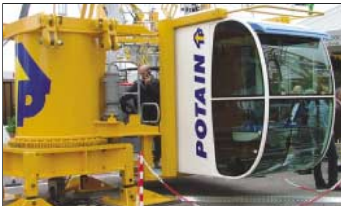
Potain's new tower cab as fitted to the new MDT 98 unit.
