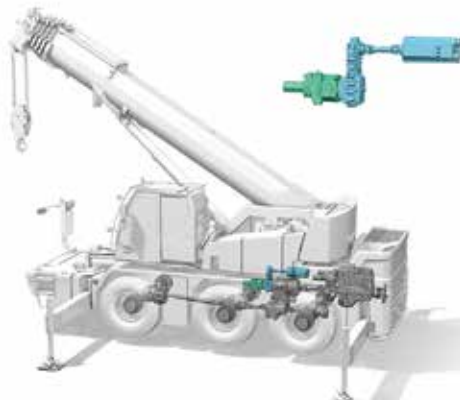
A diagram showing how Liebherr's electric system connects to the crane's transmission
